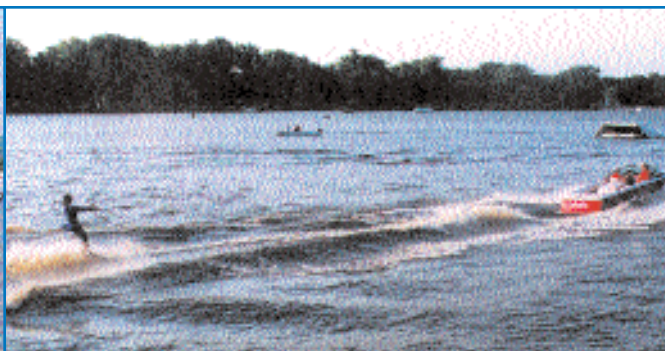
This speedboat pulling a skier travels at "transitional speed." Notice the Kelvin wake behind the boat. The skier leaves a complex wake, too.
