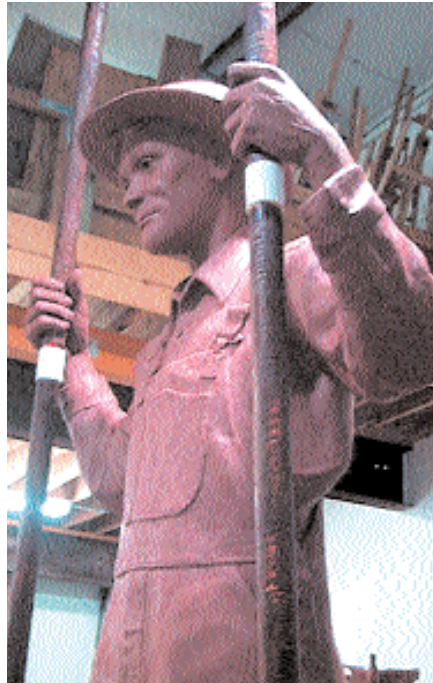
The bronze sculpture is being made from a cast taken of a full-size clay sculpture. (Photo courtesy of the Muscatine History & Industry Museum.)
